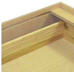
Particleboard construction (back detail)
